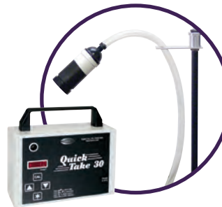
Use a QuickTake 30 with Asbestos cassette mounted on tripod – see page 104
