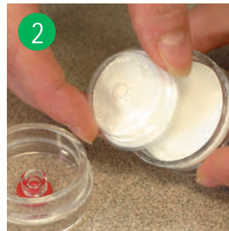
2 Weigh Accu-CAP and insert in cassette.
