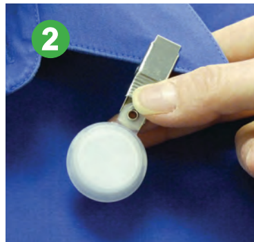
Clip in worker's breathing zone to sample.
