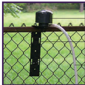
Rain cover protects sampling head
