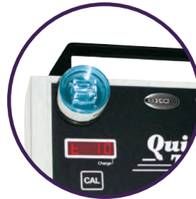
QuickTake 30 with VersaTrap cassette mounted on pump inlet – see page 114
