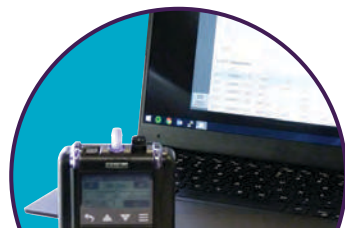
BLE communication with PC and DataTrac Pro Software for pump and data management
