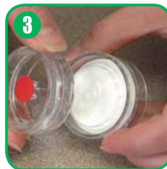
3 Complete cassette assembly. After sampling, remove Accu-CAP from cassette and weigh.
