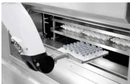
Robotic system for the loading vials in Nest.
