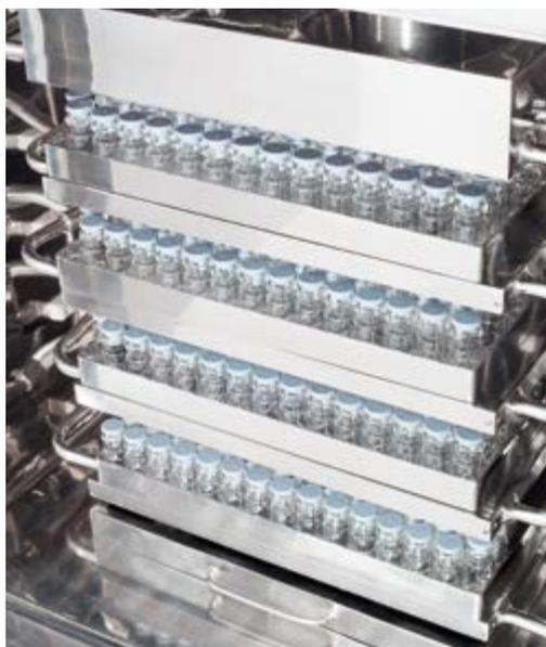
Vial batch ready for freeze drying.
