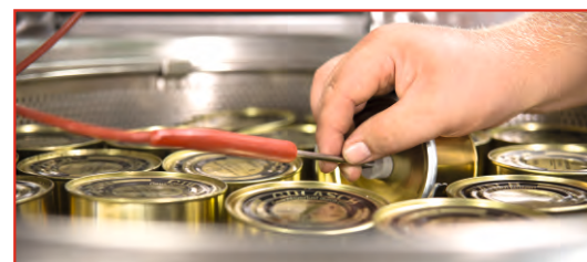
The cooking process is measured in the product using a pointed probe.
