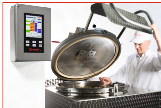
The operating panel for the cooking process control is separately fitted and supplied, saves all the information and offers facilities for contactless data exchange.
